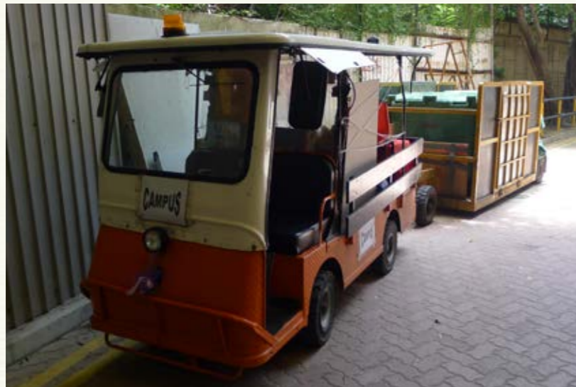
Electric Vehicle Replaced Traditional Diesel Vehicle for the Delivery of Municipal Waste to Reduce Air Emissions 以電動車取代傳統柴油車運輸廢物，減少廢氣排放
